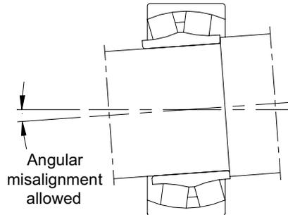
Figure 1 A Spherical Roller Bearing on a Shaft.
